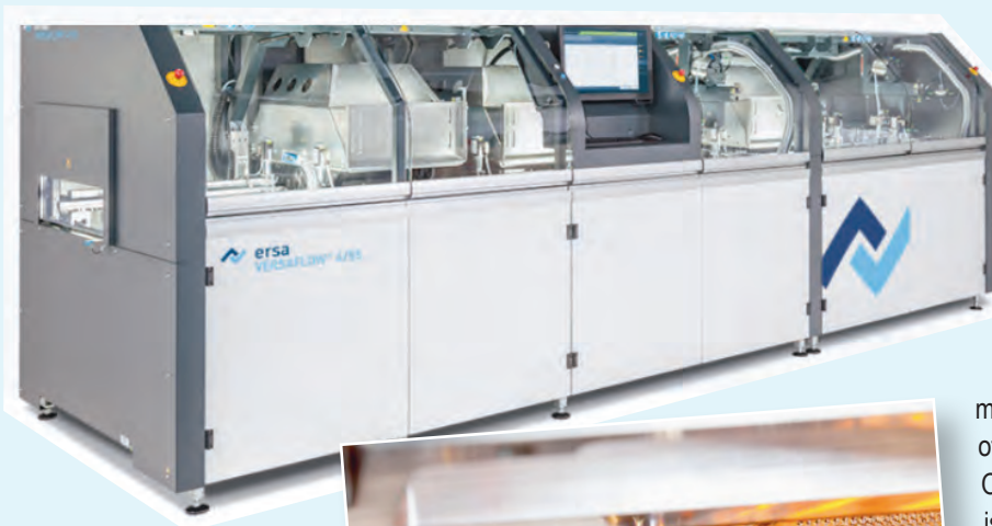
Selective Soldering with VERSAFLOW 4/55 gives us the highest flexibility for PCBAs.
